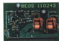
80.01.63 On-board mains voltage identification system
